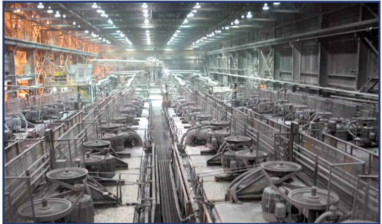
Figure 42b. Flotation tanks in the mill separate a detergent “suds” rich in metal particles from other fine rock particles. Sand and mud are pumped as a slurry by pipe to a storage reservoir. (Photo by R.Turner)
