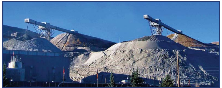
Figure 40. Conveyor belts carry football size blocks of ore from the pit to stockpiles (centre) at the mill (lower left), ready for processing. (Photo by R. Anderson)
