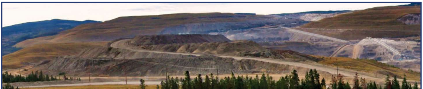
Figure 44. A view of the active mining area and surrounding reclaimed mine dumps. The reclaimed mine dumps are golden brown grasslands that have been smoothed, covered with soil, and planted with grasses. The conveyor belt is the white diagonal line and transports ore from the mine pit (lower right) to the mill (centre and hidden behind active rock waste dumps). (Photo by R. Anderson)
