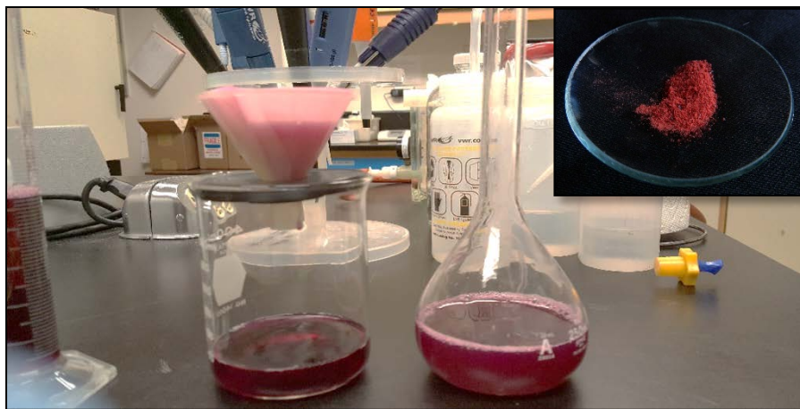
Figure 3.4 - The saturated ammonium Reinecke salt solution
