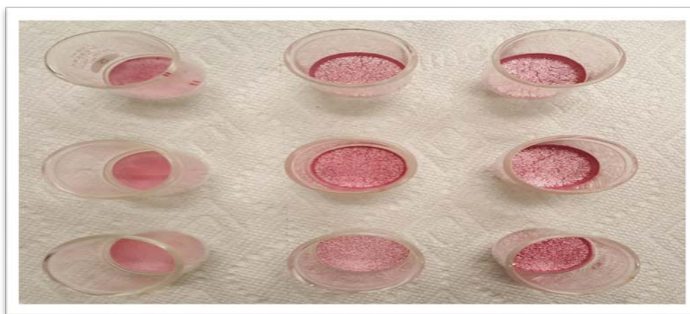
Figure 4.26 - Collected choline reinecke precipitates
