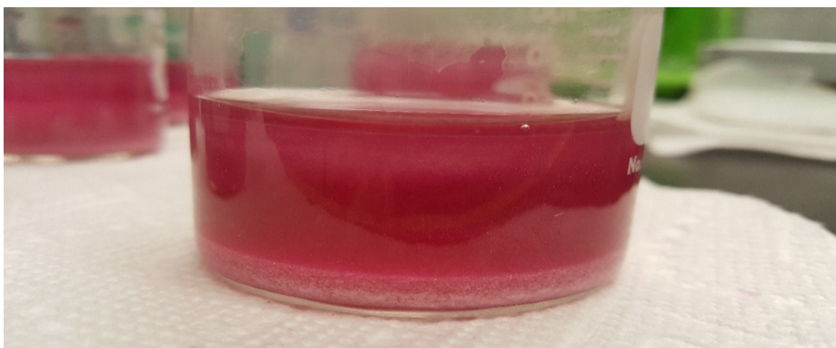
Figure 3.5 - Formed choline reinecke precipitates in the mixture
