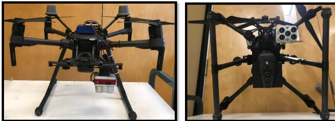
Figure 2.3. Drone (UAV currently known as RPA) equipped with a high resolution multispectral camera with a blue (475 nm center, 20 nm bandwidth), green (560 nm center, 20 nm bandwidth), red (668 nm center, 10 nm bandwidth), red edge (717 nm center, 10 nm bandwidth), near-IR (840 nm center, 40 nm bandwidth) narrow bands and thermal sensor (LWIR: 8- 14 \mu m).
