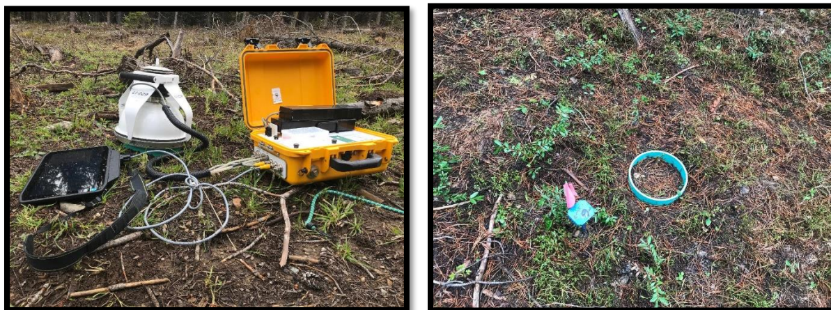
Figure 3.3: LI-COR, LI-8100A automated CO 2 soil gas flux system with a direct survey chamber ranged between 0ppm to 20,000ppm and an operating temperature range between -20°C to 45°C. A green soil Collar with a 10 cm inside and 11.4 cm outside diameter, and with 10 cm of length inserted permanently in the soil, and a minimum of 2 cm extension above the soil surface (Li-COR Biosciences 2010a).
