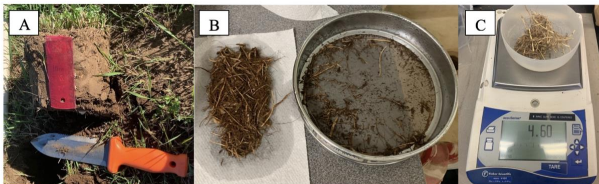
Figure 2.6: Method of root biomass collection: A) Field sample collection; B) Washing roots to remove dirt; C) Weighing washed and dried roots for final sample weight.
