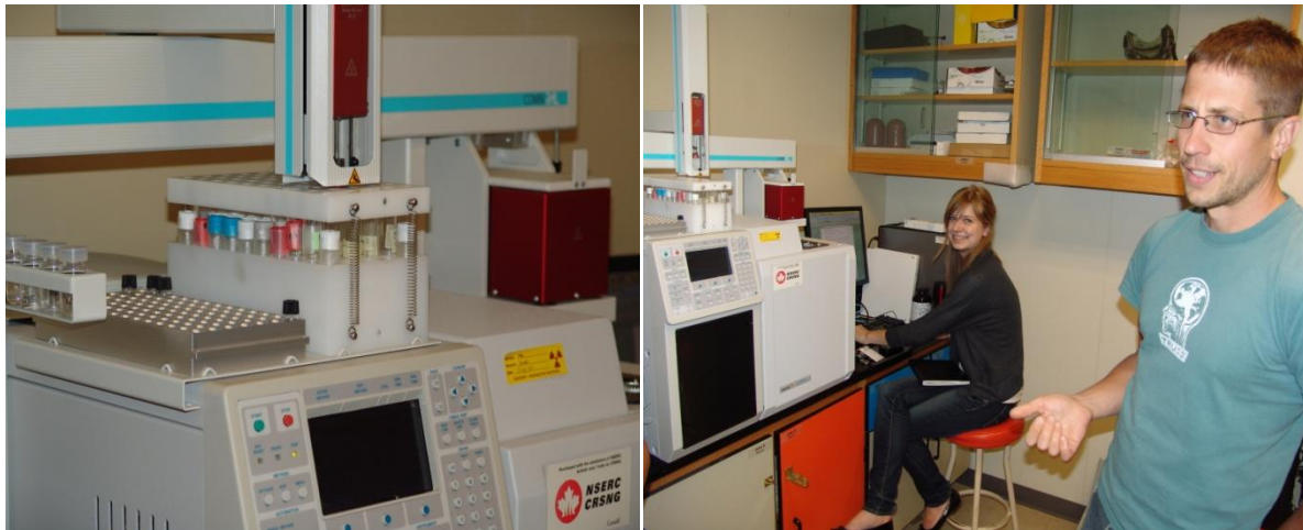
Figure 2.6. Measuring methane samples using gas chromatography.
