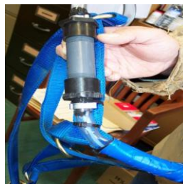
Figure 2.3. Stainless Steel capillary tubing housed in PVC tube for protection.
