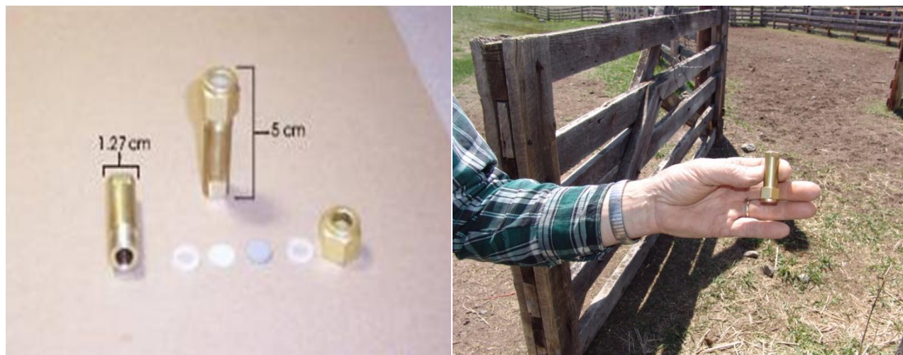
Figure 2.1. Permeation tube and components.
