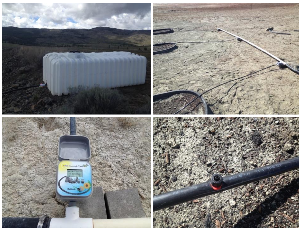
Figure 3.6. View of automatic gravity feed drip irrigation system installed at the Historic Afton Tailings Storage Facility research site in 2015. A 2000-gallon water tank elevated on the tailings dam (top left), 3-way independent water delivery system (top right), low pressure automatic irrigation timer (bottom left) and ½ gallon/hr. drip nozzle (bottom right).
