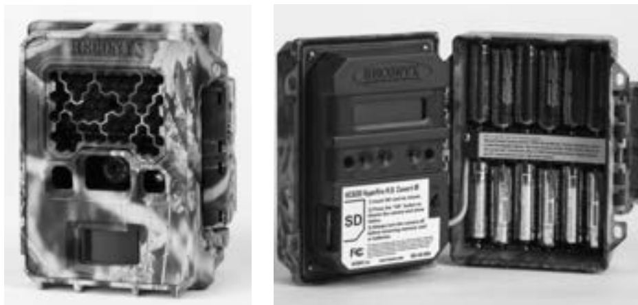
Figure 2-12 Reconyx HC500 HyperFire Semi-Covert Camera (Reconyx, 2013).
