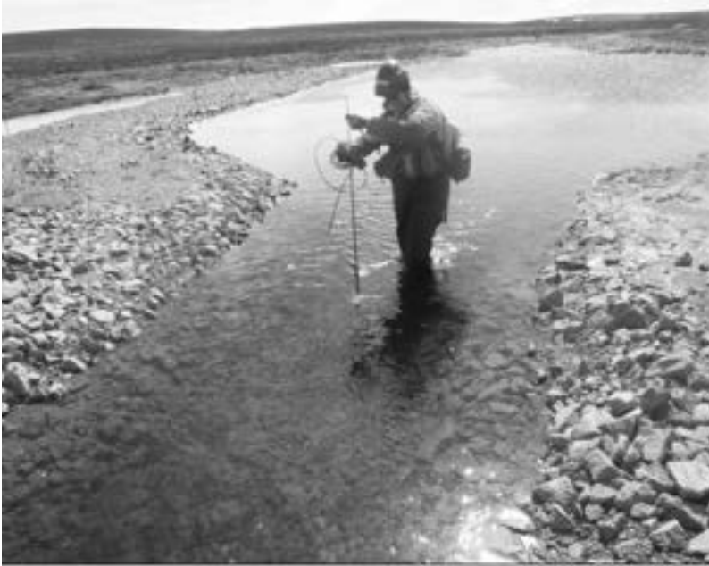
Figure 3-2 Author measuring the velocity and depth as part of the PSD monitoring program, June 4, 2014
