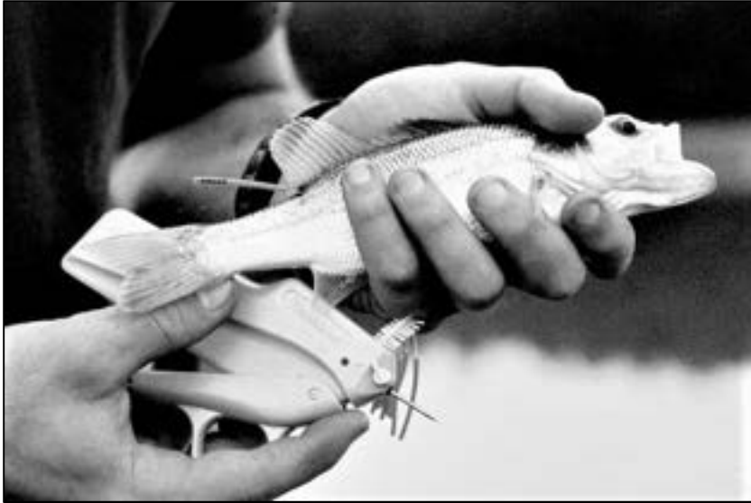
Figure 2-9 Example of Floy tag and tagger (Forestry Suppliers, 2014).
