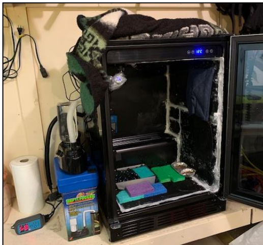
Figure 2.5. A modified beverage cooler was converted into an environmental chamber for the bat hibernation experiment. The temperature and humidity were controlled by a thermostat and reptile humidifier, respectively. Humidity was monitored with a sensor to
