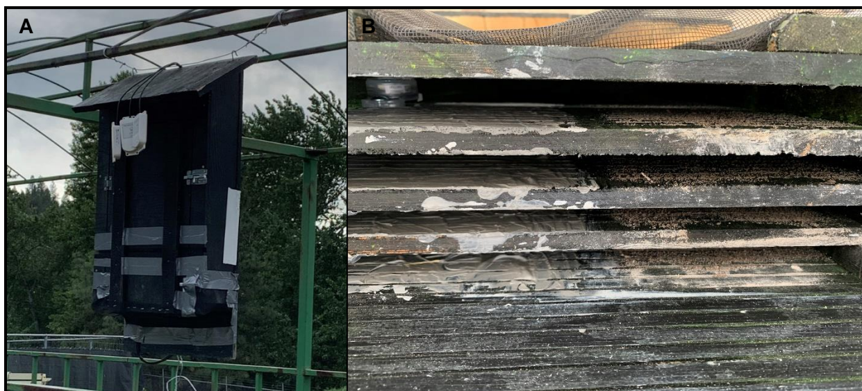
Figure 2.3. A. Four-chamber bat box hanging off the ground and away from our captive bat enclosures. B. Clay paste application (left), powder application (right) within the four-chamber bat box.
