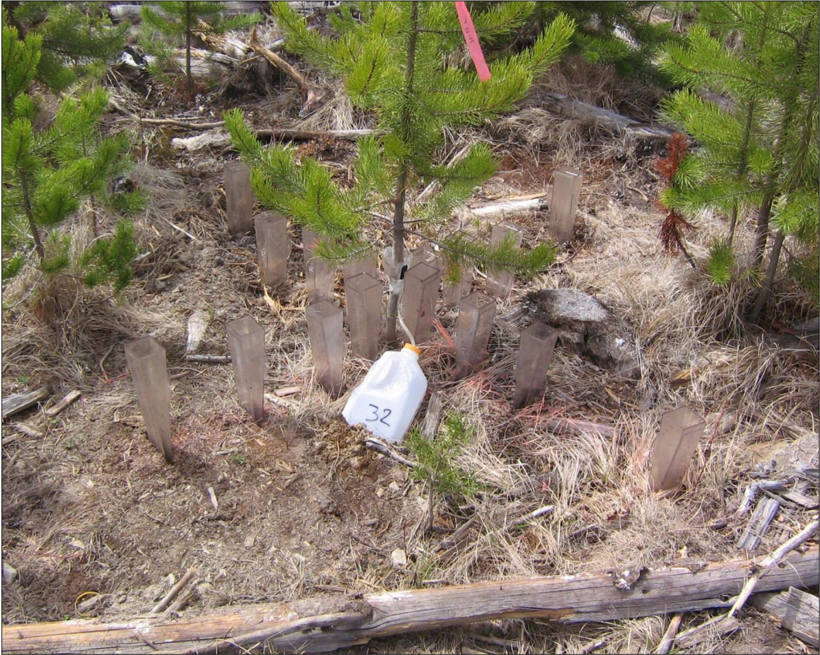
Figure 3.6: Stemflow and throughfall collection system for one of the selected study trees.
