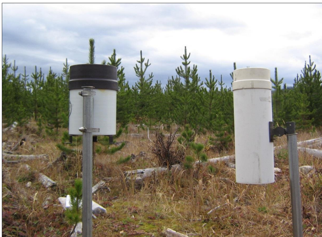
Figure 3.4: The Onset ® tipping bucket rain gauge (left) and Meteorological Service of Canada Type-B rain gauge (right) used in this study
