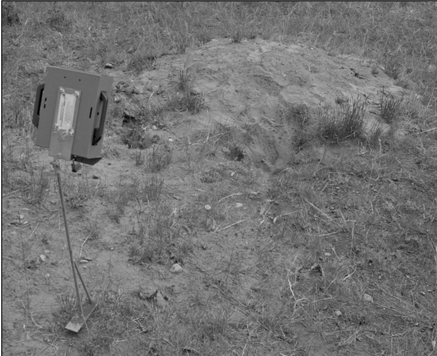
Figure 2.4. Remote infrared motion camera housed in security box attached to stand deployed at badger burrow.
