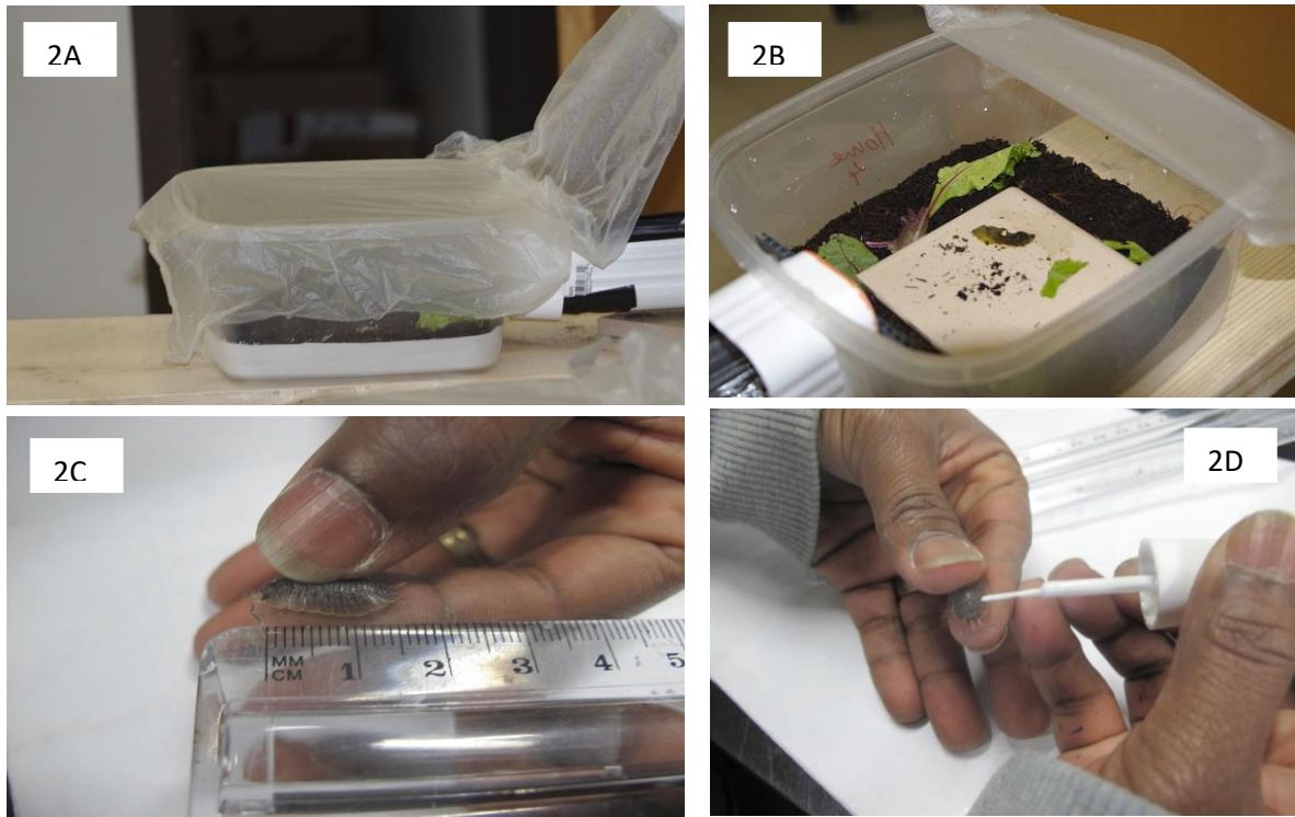
Figure 2-2. Construction of habitat containers and connection corridors: a pair of plastic sandwich containers were connected to one another via a PVC gutter pipe; the floor of each container and the corridors were layered with 2.5 cm Plaster of Paris to serve as substrate (2A). The habitat containers also were provisioned with \approx 1 cm of sterile potting soil and a raised ceramic tile that provided cover (2B). Each and every individual's size was measured (2C) and individuals were provided with a distinct mark (2D) to be identified during the experiment.
