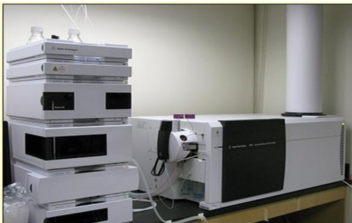
Figure 3.5. Liquid chromatography-mass spectrometer (LC/MS) used in the experiments
