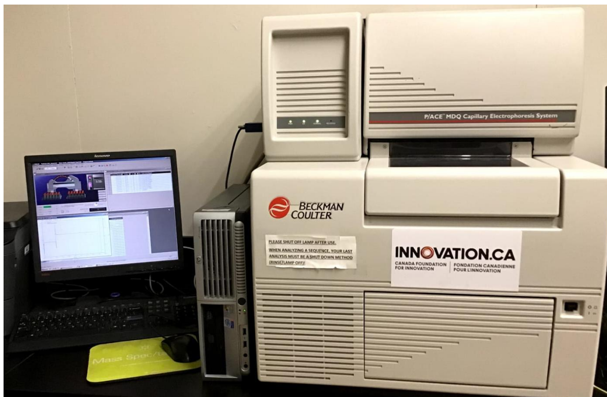
Figure 3.1. Picture of capillary electrophoresis system used in the Donkor research laboratory.
