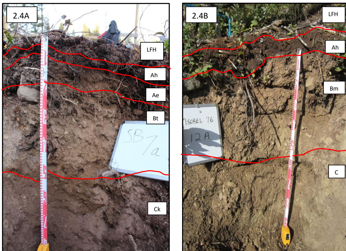
Figure 2.4: Soil profile of pit 7, face 'A' (2.4A): representative of a Orthic Gray Luvisol also found in pits 2, 5 and 17 at the Isobel site. Soil Profile of pit 12, face 'A' (2.4B): representative of an Orthic Eutric Brunisol discovered in the remaining 16 soil pits.
