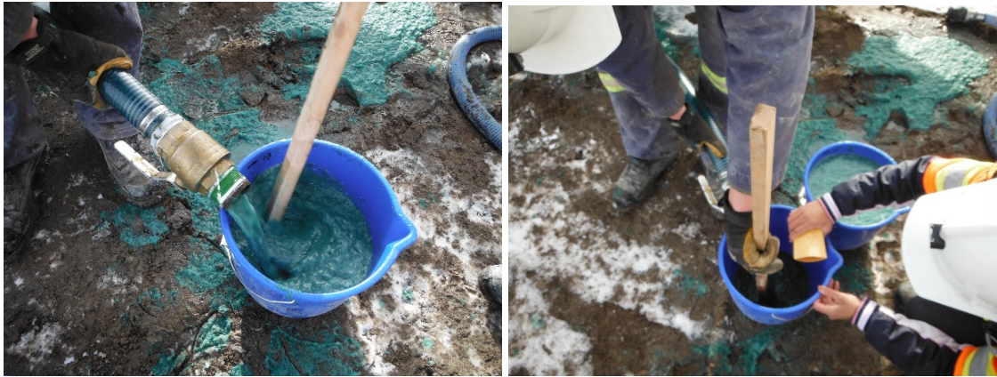
Figure 3.3: Hydro-seeding sites on stockpiled topsoil at New Gold's New Afton Mine Site. Buckets were marked at the 12 L line and then filled with hydro-slurry (left). In preparing the buckets for spreading, ½ of the seed packet (control seed packages with no seed and packages with seed) were emptied into each bucket and stirred to mix thoroughly before being spread on the appropriate treatment plot (right).
