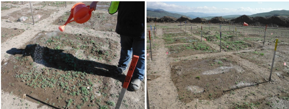
Figure 3.5: May and June watering of site preparation and seeding study at New Gold's New Afton Mine site. Watering was completed by hand using watering cans with dispenser heads (left). All plots were watered with 4\text{mm}/\text{m}^2 twice a week. The right figure shows a plot with standing water which was allowed to seep into the soil before more water was applied.
