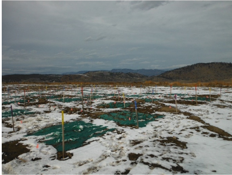
Figure 3.4: Stockpiled topsoil at New Gold's New Afton Mine site after the grid was seeded. Treatment plots were either raked, hydro-slurried, raked x hydro-slurry, or had no manipulation and each of these factors was either with or without seed. Seeding took place in November 2012.
